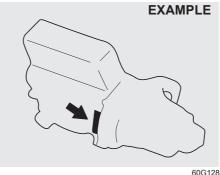
The engine serial number is stamped on the cylinder block as shown in the illustration.
