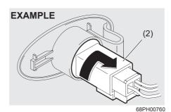
2) Turn the bulb holder (2) clockwise and pull it out from the light housing.
