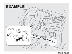
You can unlock the lid by pushing the trunk lid unlatch button (2).
