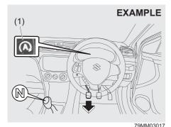
2) Manual transaxle - When decelerating at approximately 3 km/h or below with the clutch pedal depressed and the gearshift lever shifted to "N", and then release the clutch pedal, the engine will stop automatically.
