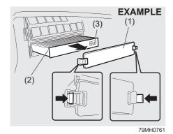
2) Remove the cover (1) and pull out the air conditioner filter (2).
