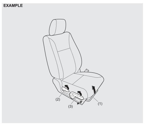
**Seat position adjustment lever (1)**Pull the lever up and slide the seat.
