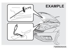
While holding the hood, pull the prop rod out from the holding clip, then insert the end of the rod into the designated hole.
