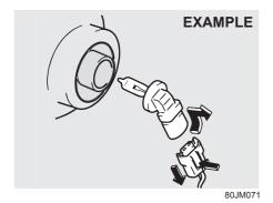
Disconnect the coupler by pushing the lock release. Turn the bulb holder counterclockwise and remove it. Rear Combination Light Halogen rear combination light
