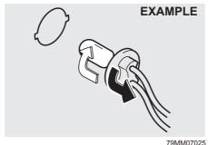
To remove a bulb holder from a light housing, turn the holder counterclockwise and pull it out. To install the holder, push the holder in and turn it clockwise.
